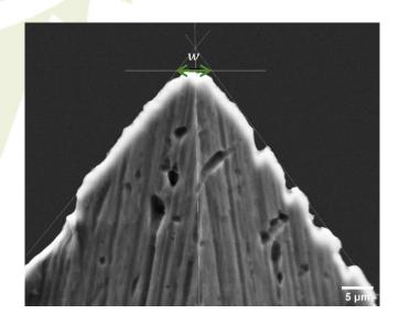
unavoidable during an injection, a needle is therefore deemed blunt if  $w>30\mu m$ , as using such a needle would inevitably cause more damage than necessary.
