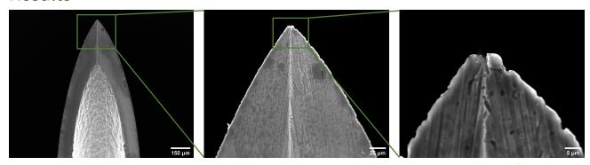
A single needle is shown above at increasing magnifications. A magnification of 5000X reveals far more detail than optical microscopy would be capable of. The porosities in the metal are clearly visible, as well as the lines where the tip was ground to a point.
