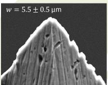
Most needles appeared sharp, with measured tip widths between 5 – 10 μm.
