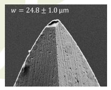
Two needles were slightly damaged, with tip widths greater than 20  $\mu$ m.
